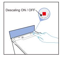
2.Press the descaling button and start the water tank drainage; the nozzle will self- clean during the drainage process, accompanied by drops beep. If misoperation, the product can be used normally after power off and restart.
