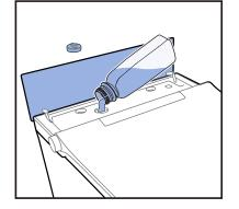
3.After the water in the tank is drained out completely; add the scale remover (recommend coffee machine scale remover); the maximum capacity is 250ml.
