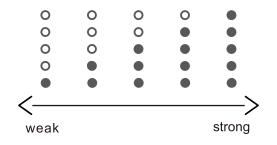
Press "  $\land$  " to increase the water pressure. Each time you press it, it increases by 1 grade up to the highest grade. Press "  $\lor$  " to decrease the water pressure. Each time you press it, it decreases by 1 grade up to the lowest grade.
