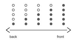
Press "  $\land$  " of the "Nozzle position adjustment", the nozzle extends forward, and each time you press it, it increases by 1 grade up at the highest grade. When you press "  $\lor$  ", the nozzle retracts backward, and each time you press it, it decreases by 1 grade up to the lowest grade.
