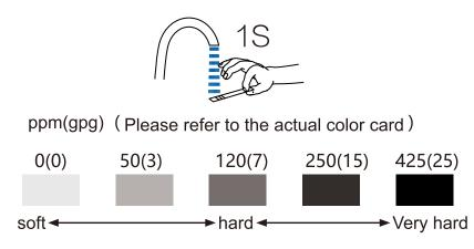
Measure the water quality at the installation site, immerse the reaction area in the test solution for 1 second, and remove excess water drops;
