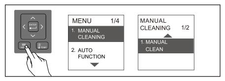
2. Activate the nozzle cleaning according to the above operation on the back of the remote control. The nozzle is extended without water.
