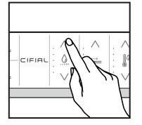
Under lady washing, press "  $\wedge$  " of " Water pressure adjustment " to increase the water spray intensity; press "  $\vee$  " to decrease the water spray intensity.
