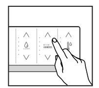
During rear washing, press " $\wedge$ " of "Nozzle position adjustment" to move the nozzle forward; press "  $\vee$  " to move the nozzle backward.
