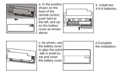
Try to operate the remote control. If the state light of the remote control lights up with the button, the battery will be installed successfully. If the remote control is not available, please check whether the battery is charged and correctly installed. If the battery runs out of power, you can change the new battery follow above.
