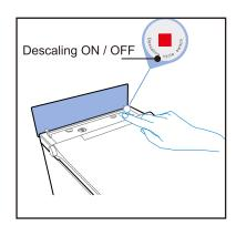
4.Press the descaling button again to start the descaling cycle.
