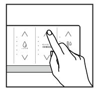
During lady washing, press "  $\wedge$  " of " Nozzle position adjustment" to move the nozzle forward; press " $\lor$  " to decrease the water spray intensity.
