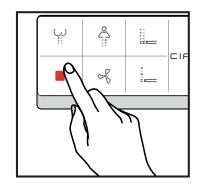
Press the "Stop" button to stop or wait for 3 minutes to stop automatically.
