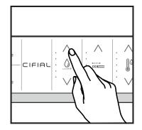
During rear washing, press "  $\wedge$  " of "Water pressure adjustment" to increase the water spray intensity; press " $\checkmark$ " to decrease the water spray intensity.
