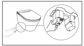
4.Water quality conditions are different in different regions. P leas e c lean the water tank regularly. Blocking of dirt may cause the water flow to decrease. (Recommended once every 2-6 months). Drain the water in the water tank by pressing the drain button under the water tank. (As shown in FIG).
