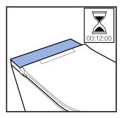
5.During the descaling process, the status lamp flashes. After 9 minutes, the descaling cycle is completed and the status lamp comes back to normal.
