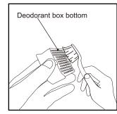
③ . Use a toothbrush or a brush to clean the bottom of the deodorant box until there is no dust or paper dust.
