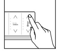
During lady washing, press " $\wedge$ " of " Water temperature adjustment" to increase the water temperature; press "  $\vee$  " to decrease the water temperature.
